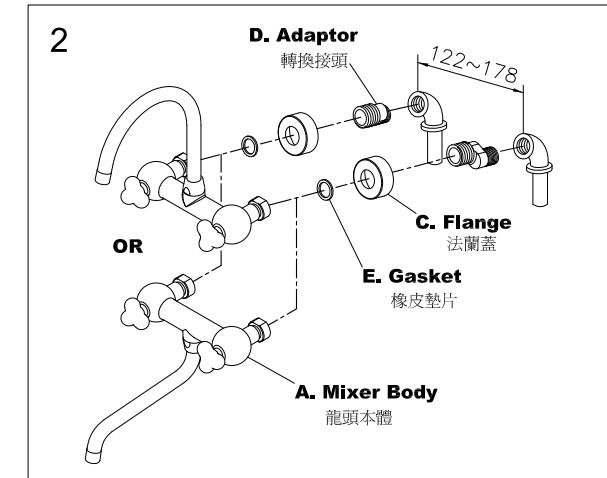
NOTE: The available distance between two centers of wall water-outlet can be 122~178mm as Fig.2 shown.
