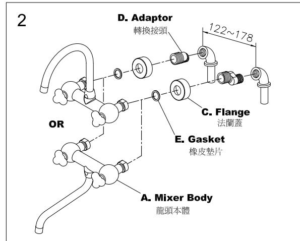
NOTE: The available distance between two centers of wall water-outlet can be 122~178mm as Fig.2 shown.
